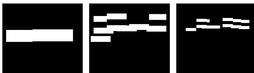
Fig. 11. Result of primitive pattern detection on the radiograph shown in Fig. 10 by means of the multi-scale image analysis using relevance function. A set of artificial binary primitives has been used.
